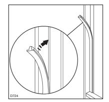
Apply covers (B) on joint cover lugs and into hinge holes.
